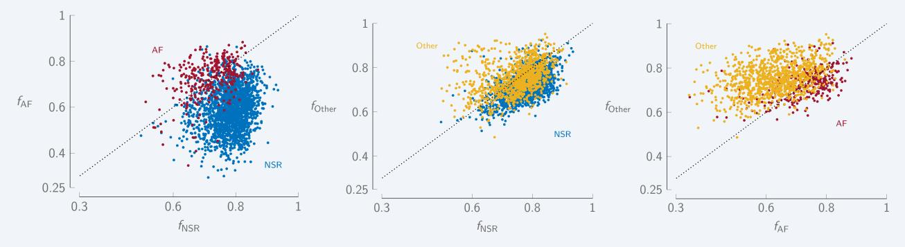
A clear separation between the AF class and normal class (NSR) shown by the morphological features on the PhysioNet/Cinc challenge 2017 dataset.
